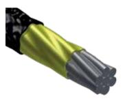
Supplementary corrosion protection layers are guaranteed with the use of galvanized wires, a thin layer of corrosion inhibitor (wax or grease) and a co-extruded hdpe coating.
