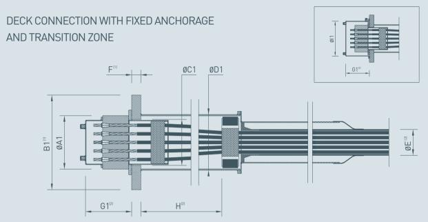
Main dimensions (using steel strand diameter 15.7 mm and grade 1 860 MPa)
